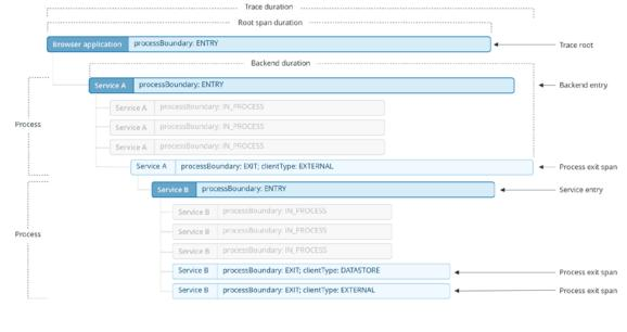
A distributed trace has a tree-like structure, with "child" spans that refer to one "parent" span. This diagram shows some important span relationships in a trace.
